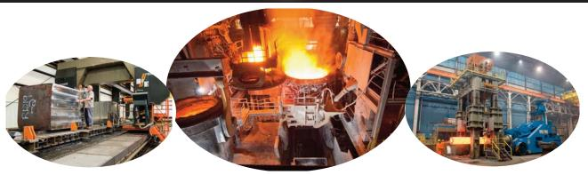
**Ellwood Specialty Steel** is a fully integrated producer of a wide range of specialty tool steels. Our ExELL grades are made with advanced ASEA-SKF steel making capabilities which include an ultra high powered electric arc furnace with subsequent state-of-the-art ladle refining and vacuum degassing equipment for the most complete and modern ladle metallurgy technology.
